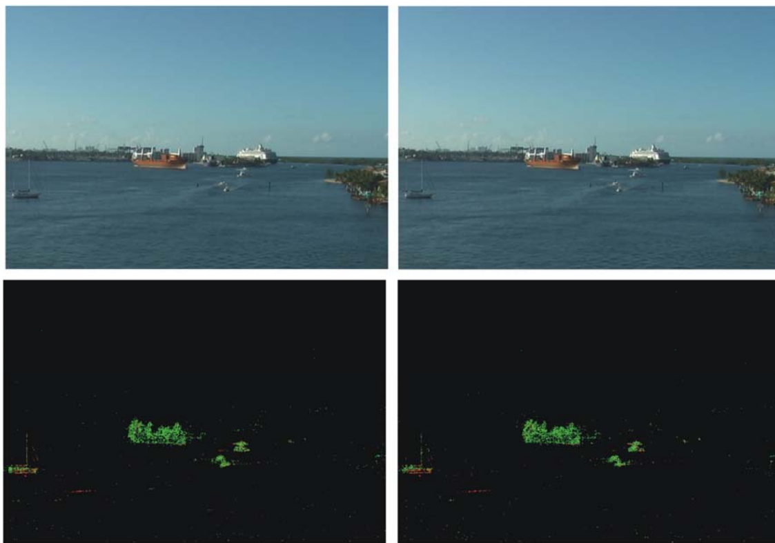
Figure 4 Two consecutive frames from a test sequence (top) and the segmentation result (bottom).
